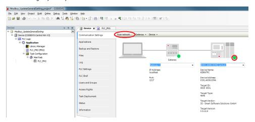
• Insert an Ethernet adapter in the device tree and specify the interface to be used.
